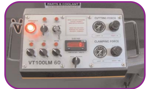
Console Pivots from Front to Right Side of Saw
